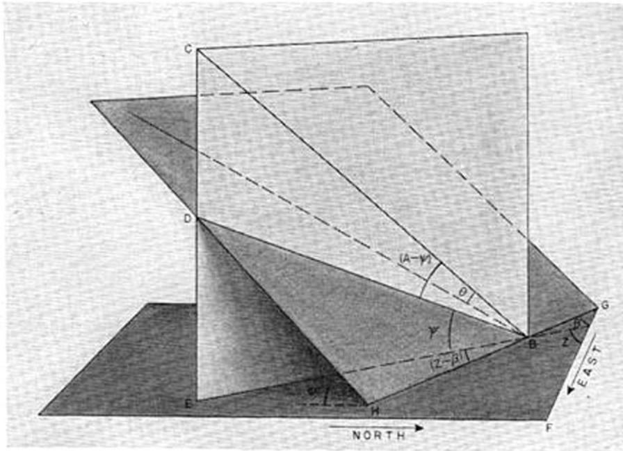
FIGURE 4.—Diagram from which the theoretical intensity of solar radiation on a tilted plane may be determined.
