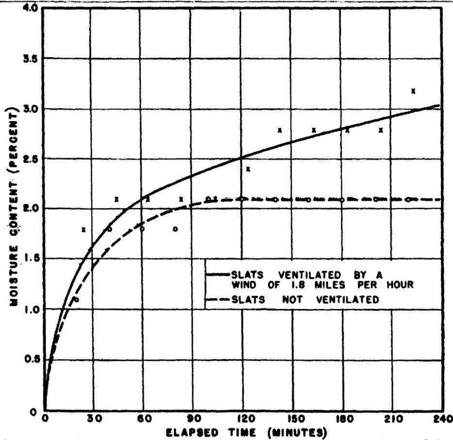
FIGURE 10.—Curves showing effect of wind on rate of gain of moisture by wood slats initially oven-dry and exposed to radiation of 1.76 calories per square centimeter per minute. Relative humidity during test, 62 percent; air temperature, 82° F
