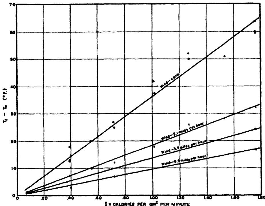
FIGURE 6.—Relation of radiation intensity  $I$  and wind velocity  $V$  to difference between fuel temperature and air temperature  $T_f - T_a$ , as established experimentally with the artificial-sun apparatus.
